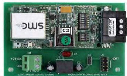
Figure 12. BMS System Interface Module
