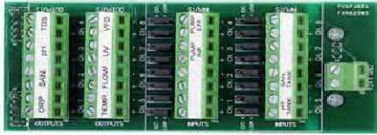
Figure 9. 4-20mA Expansion Card
