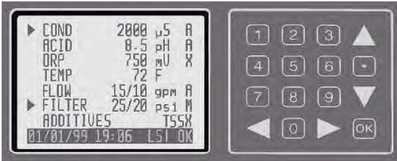
Figure 1 - Control Panel of CT6000
