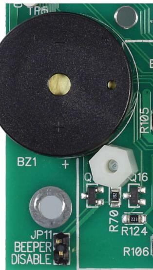
The PC3000, PC5000, 5100, PC6000, PC7000 and PC7100 series beeper is located in the lower central area of the board. It may be disabled with JP13.
