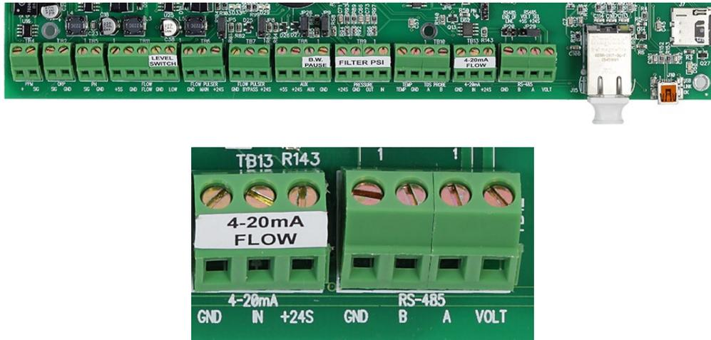
**Figure 45.** 4-20 mA Flow Meter Connections to PC 3000, PC 5000, pc 5100, PC6000, pc7000and PC 7100
