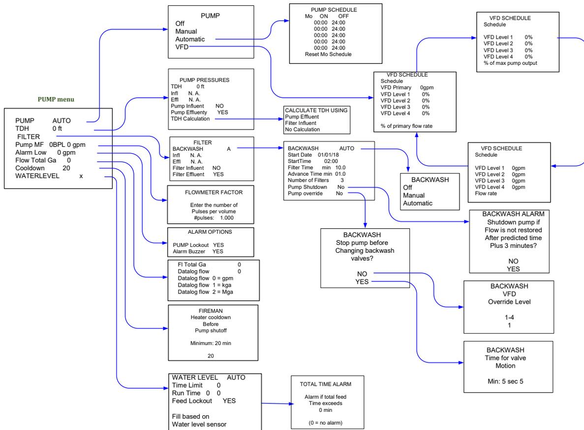
The flow meter factor is calibrated by entering the K-factor provided by the sensor manufacturer. These values correspond to the number of pulses per unit of volume in gallons or liters, which are given by the sensor manufacturer.
