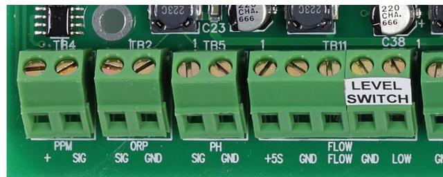
**Figure 53.** Level Switch inputs (PC 3000 and above)
