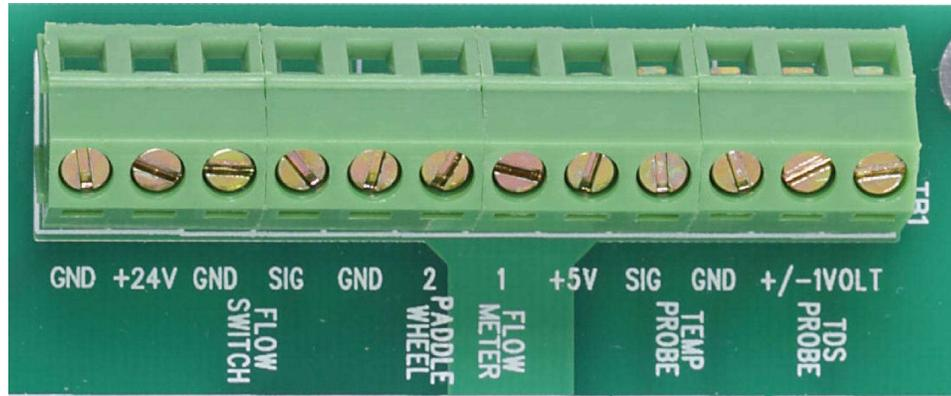
**Figure 44.** Connections to PC2100 (Power supply board)
