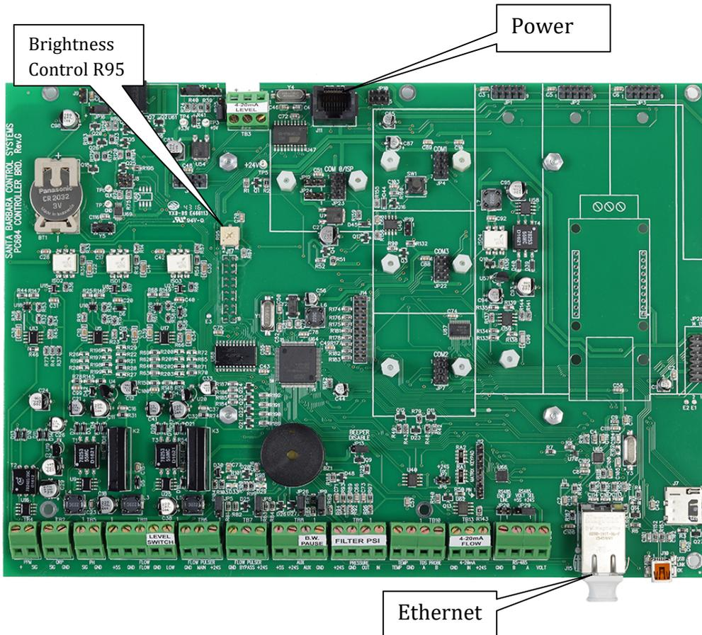
**Figure 11. PC 604 CPU Board**
