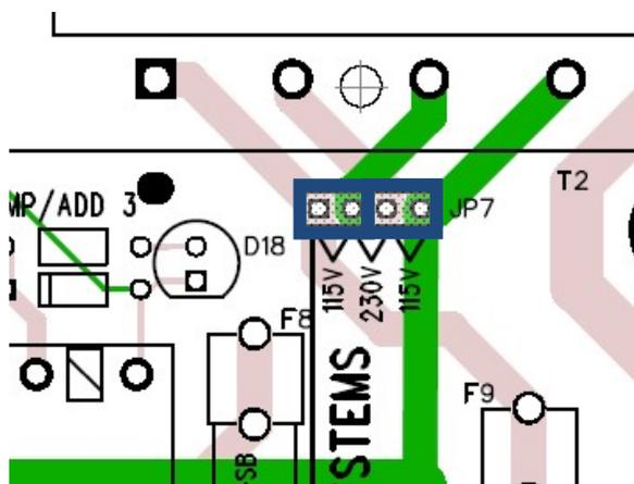
**Figure 15.** Voltage Selector Jumpers set to 115 volts (2 jumpers)
