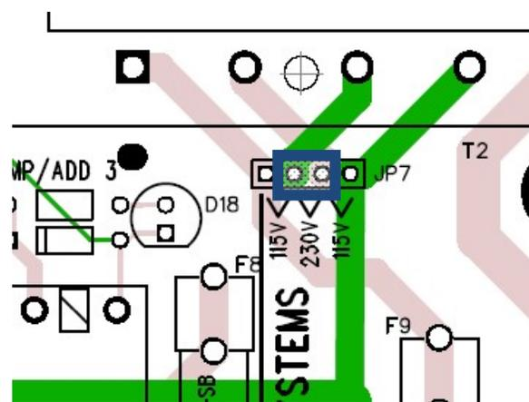
**Figure 16.** Voltage Selector Jumper set to 230 volts (1 jumper in center) 110v both (2) jumpers cover 4-pins
