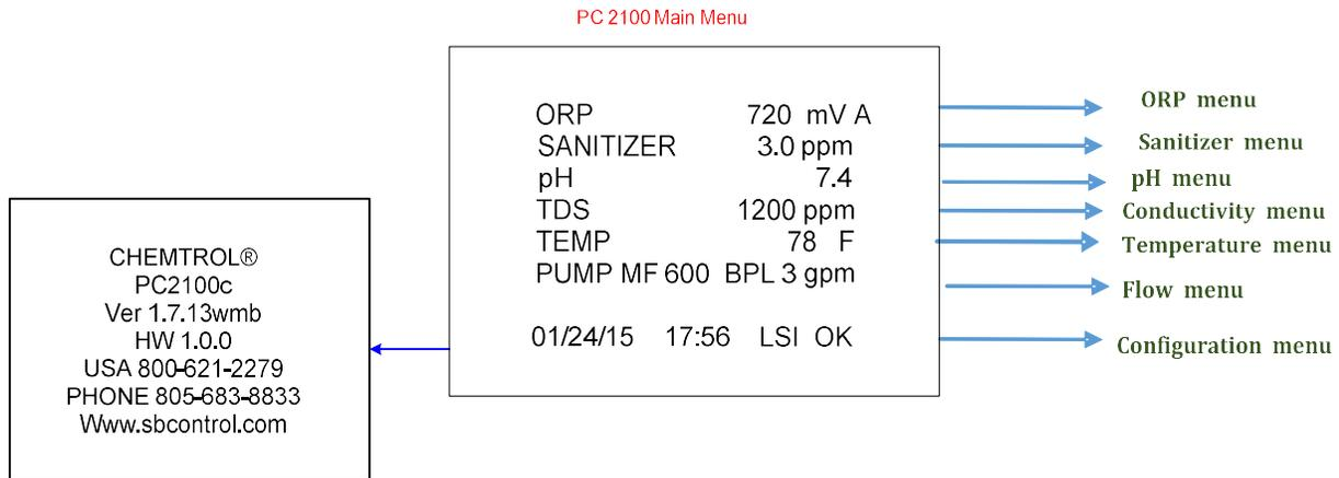
**Figure 60.** Typical Main Menu for PC 2100 series controllers
