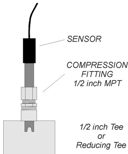
**Figure 29.** Sensor Installation
