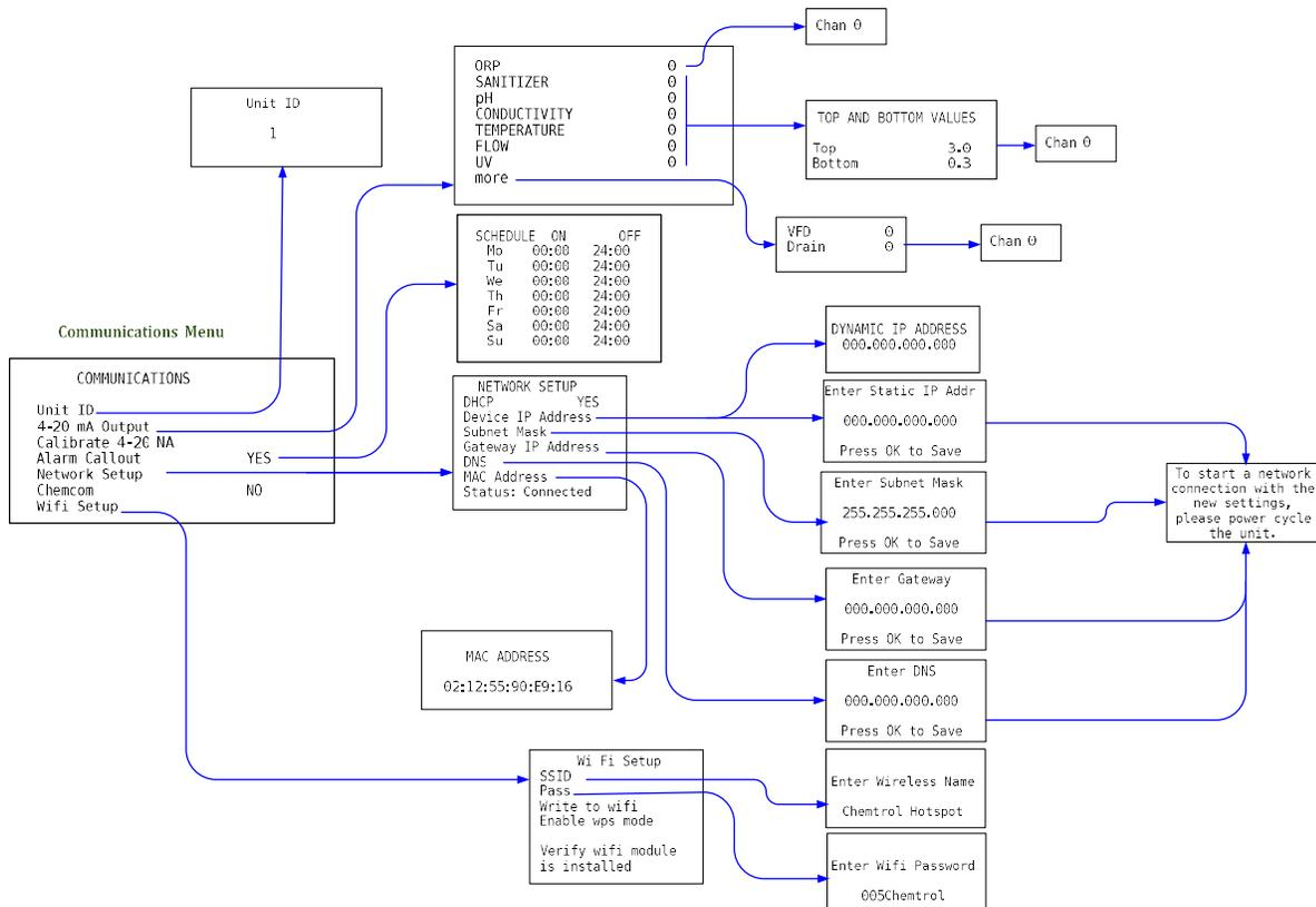
The Communications menu is used to set the Unit ID, 4-20 mA calibration, Alarm callout schedule, Network setup and Wifi setup.
