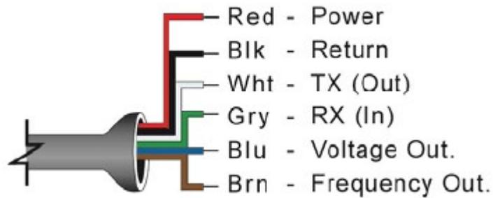
**Figure 48.** DL-10 Wiring
