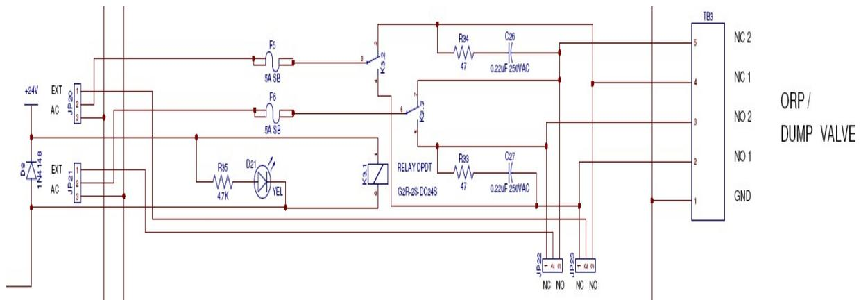
The jumpers are similarly placed on each of the relay positions. Two jumpers, labeled AC EXT control whether or not the AC power is routed through the relays. Below that are two more jumper blocks that control whether or not each relay is normally open or normally closed. Note that when the relays are used to switch AC, the normally open/normally closed terminals are directly available.
