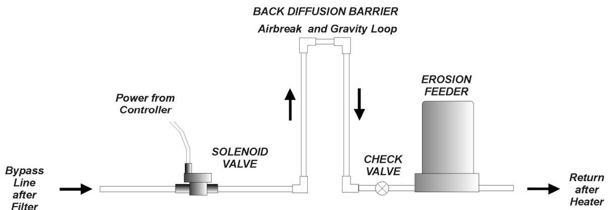
**Figure 54.** Erosion Feeder Control
