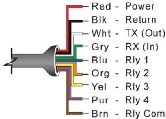
**Figure 49.** DL24 Wiring
