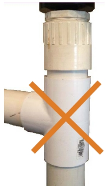
Avoid the use of a tee within the stand pipe. A tee can create false signals that will negatively effect the sensor's performance.
